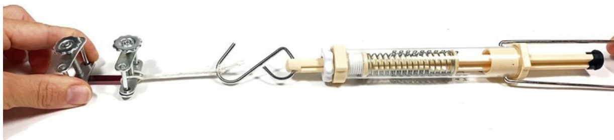
Figure 9. Tensile test setup using a spring scale.
