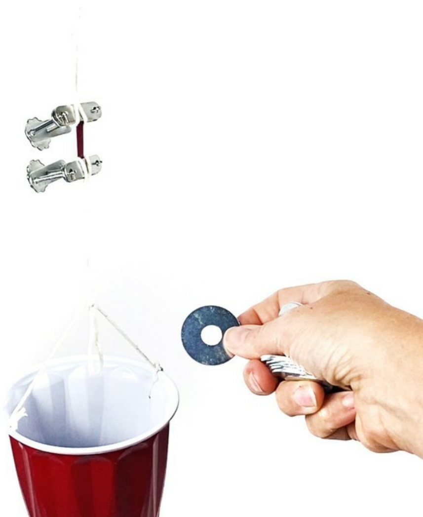
Figure 11. Tensile test setup with a cup and weight.
