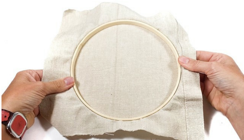
Figure 4. Prepared biofabric mold consisting of a wooden embroidery hoop and canvas.
