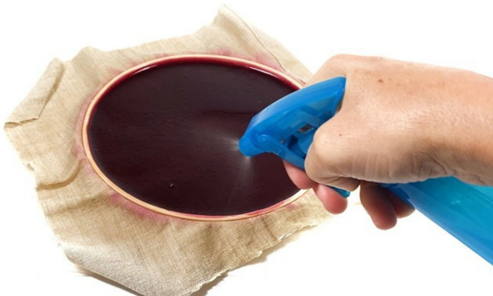
Figure 5. Spray enough calcium chloride on the alginate mixture so that the whole surface is covered.
